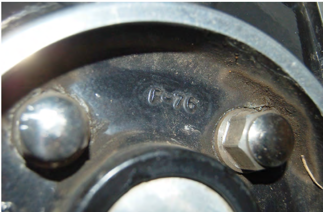
The date of the manufacture of the alloy wheels is cast into the wheel centre area.
