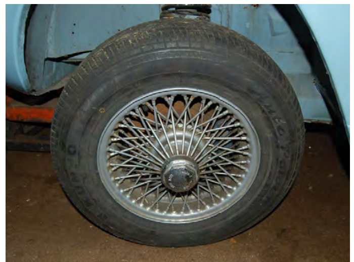
A better view showing the straight outer spoke arrangement which do not cross as they enter the hub just behind the spinner.
