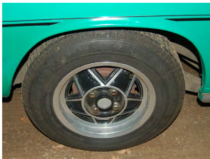
Standard alloy wheel with plain centre finisher but with replacement steel wheel nuts which were not original fitments.
