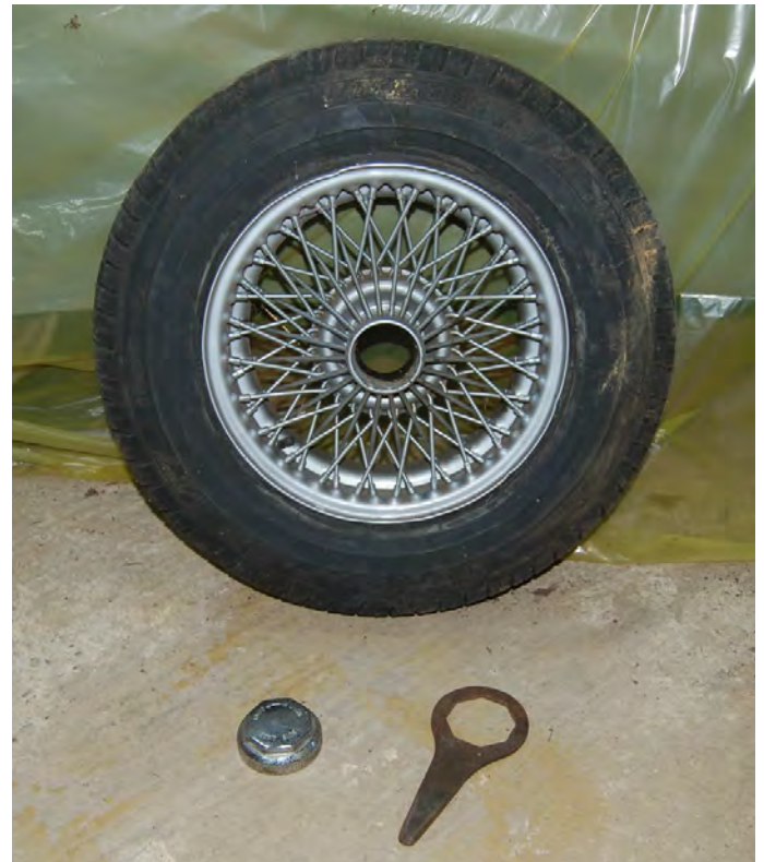
The Stag wire wheel in silver grey enamel. With original spinner design and spinner spanner
