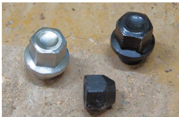
The three wheel nut patterns which were used on Stag wheels. But are the finishes correct for the steel wheel nut and the 'silver' alloy nut ?
