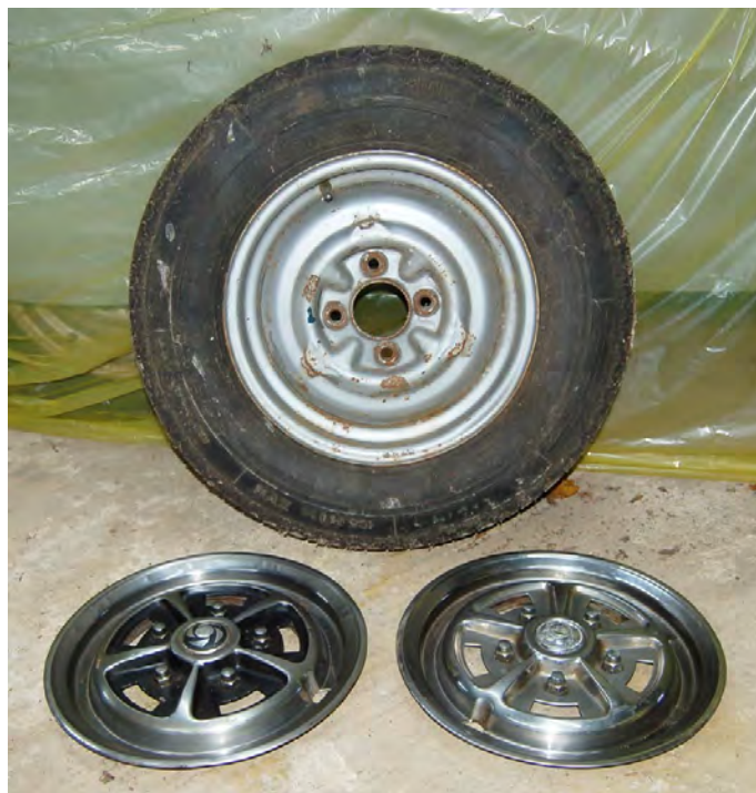
A standard Dunlop steel wheel with samples of the two designs of wheel trim – before 1973 and after 1973.
