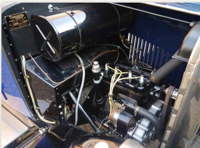
Small 832 cc sidevalve engine, nestled low in the engine bay.
