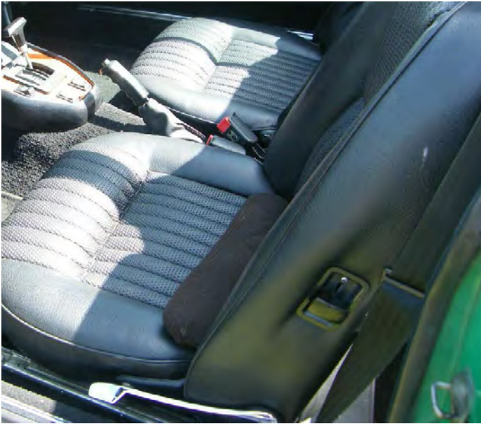
The position of the Mk2 seat release, about halfway up on the side of the seat.
