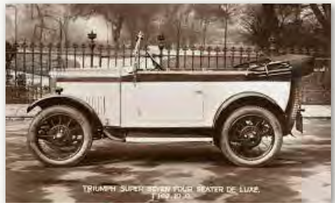
Triumph 2-Door 4-Seat Super Seven Tourer De-Luxe. Compare this with the photo of the 13/35 on the previous page and you will see how much smaller this car was (27 inches shorter in the wheelbase).
