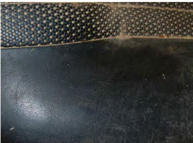
The almost smooth material of the very early seat. This is an LD7 seat.
