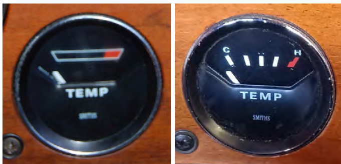
The late style gauge (left) as shown in my earlier article and the early style gauge (right) as keenly noted by Paul.
