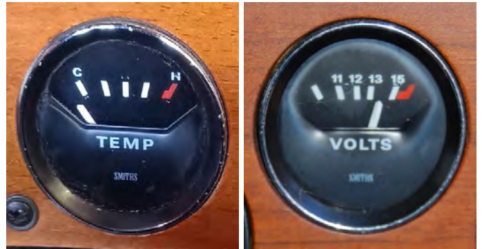
The matching temperature gauge and the voltmeter used on very early Mk2 cars. If you have an early Mk2 car, you are indeed blessed !
