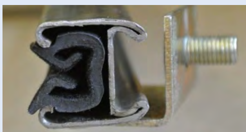
Profile too tight
