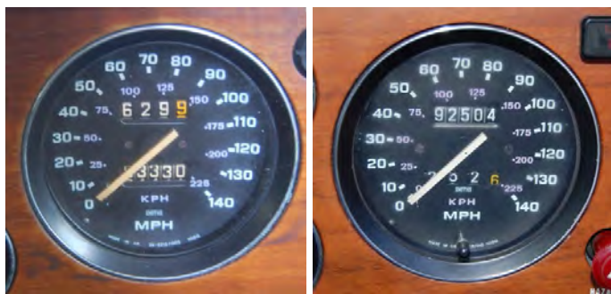
The earlier speedo (left) which Martin's car has and the later speedo (right) which was not fitted at LD 35940 but a month or so later.
