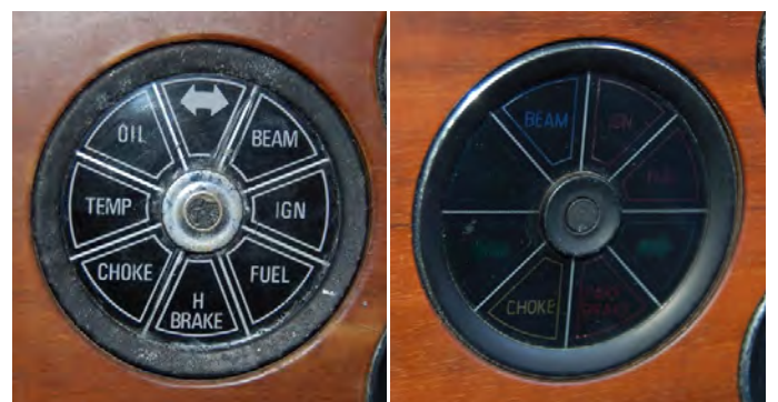
The early warning light cluster (left), and the late warning light cluster (right).
