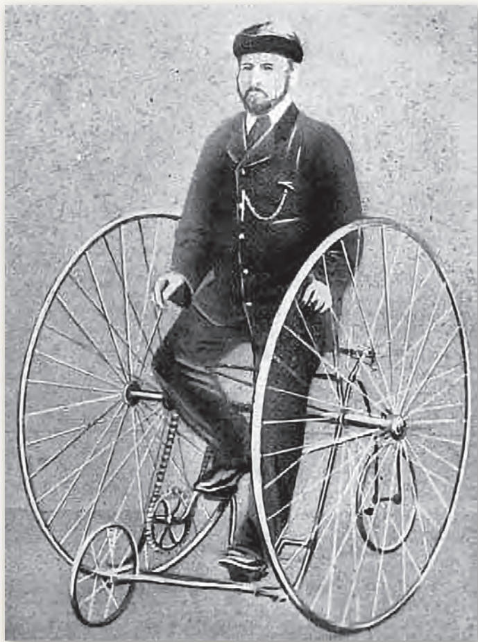
James Starley on a 'Salvo' tricycle, the first cycle to incorporate his differential gear which allowed the 'inner wheel' to revolve at a slower speed than the 'outer' when cornering (approx 1877).
