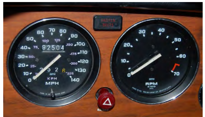
The UK hazard warning light fitting for cars after LD30001 – at the bottom of the main instrument panel.
