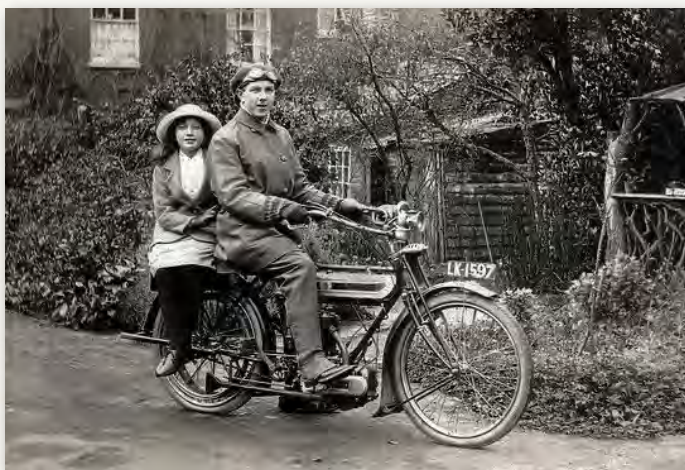
An obviously posed photo taken in 1911. The machine is still a motor bicycle with pedals to get started.
