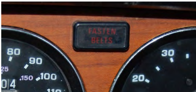
The seat belt warning light fitting for cars after LD30001 – at the top of the main instrument panel.
