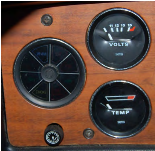
The Panel lamp dimmer is bottom left, under the warning indicator cluster.
