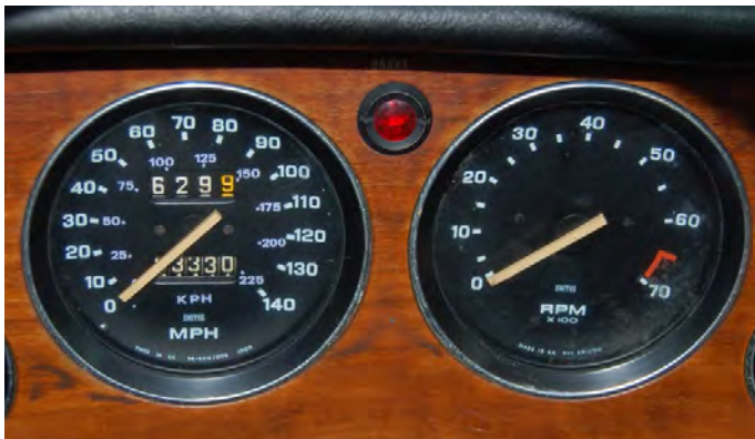
The early position of the brake line failure warning lamp – between and above the two main gauges.
