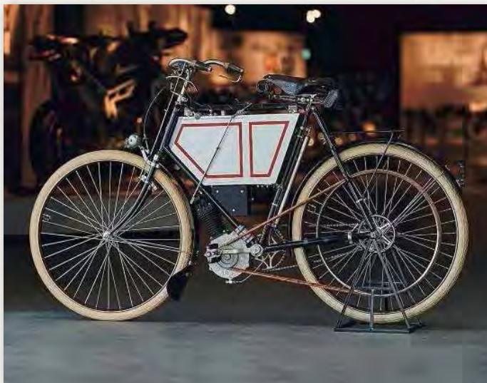
The first Triumph motor bicycle – recently discovered. Belt driven by the Minerva engine but retaining the chain drive of the original bicycle (on the other side of the 'bike').
