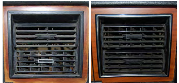
Central louvre ventilators from before LD20001 (left) and after LD20001 (right). The difference being the silver painted rim to the surround.
