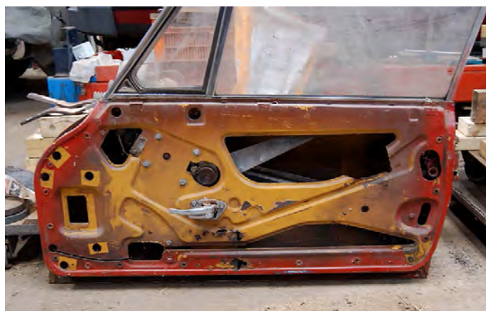
The inner framing of a later door showing the single cut out for the lift motor and the removal of the cut-out for a manual window winding handle.
