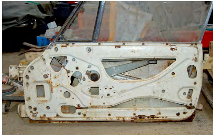
The inner framing of an early door showing the two cut outs for alternative lift motor positioning and a cut-out below these for a manual window winding handle.
