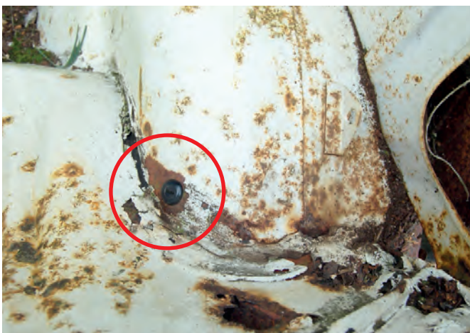
The position of the black plastic insert in a 1972 model year car – in the corner of the rear wheel arch.
