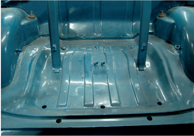
The position of the four anchor bolts in the rear floor pan in an early Stag.
