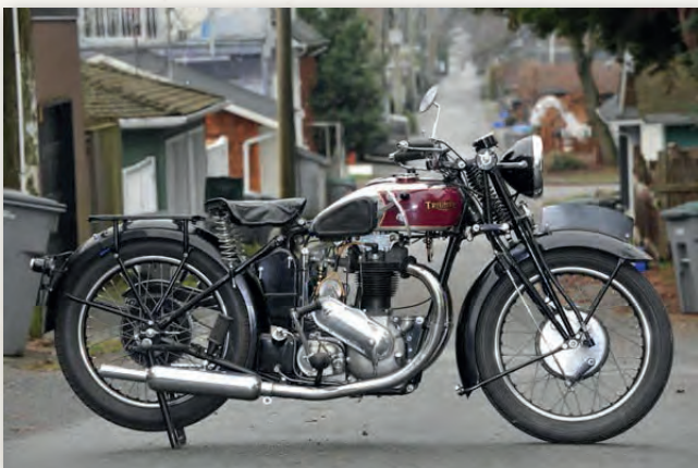
A 1935 650cc Triumph 6/1. The first British bike to have a parallel vertical twin engine.
