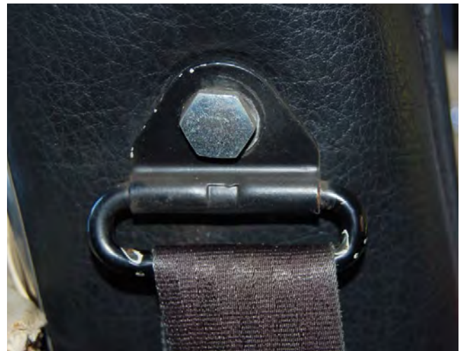
A late top seat belt fixing bracket and bolt. Note that the bracket is different to that on the early cars which just had slot cut in the bracket for the belt to pass through. This later bracket has an oval link fixed into the flat part of the bracket.
