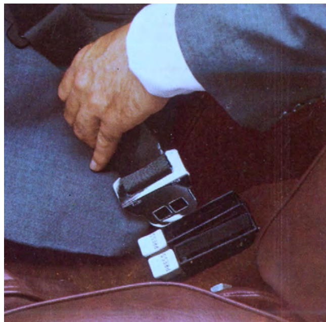
An excerpt from a 1974 advertising brochure showing an alternative seat belt catch and tongue.
