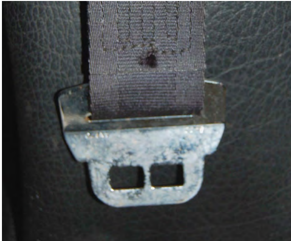
The second type of tongue, with two smaller holes. The catch on the transmission tunnel stayed the same – with a single white surround for both catches and black buttons at the front.
