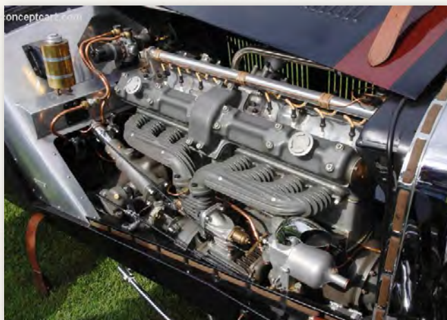
Another way of joining two 4-cylinder blocks – end to end – the camshafts and crankshaft were also in two sections.
