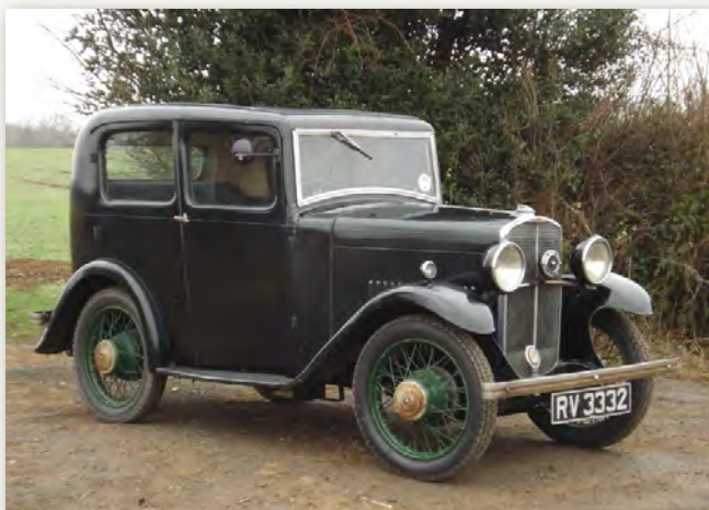
A 1933 Super Eight – a small car, but with all the extras. Note the four doors (count the hinges) but only one door handle – an interesting pillarless construction.
