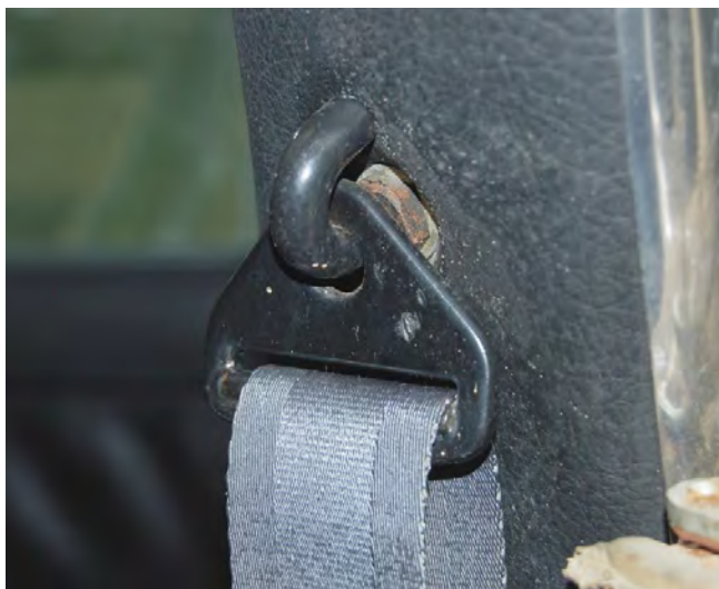
In the early Mk2 cars, the top fixing is by a hooked bolt screwed into the B-post with the hook passing through the fixing bracket
