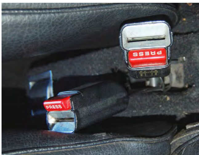
The later catches mounted to the transmission tunnel with short flat plates which allowed the catch to swivel around the bottom bolt. These were also equipped with two wires to each catch through which the seat belt warning light was activated.
