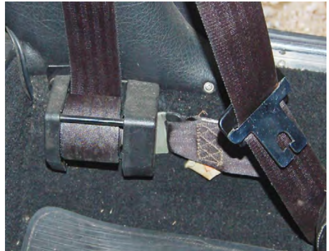
The later style of Britax inertia reel with two shaped but basically rectangular end caps but still mounted by a bolt through both the belt bracket and the inertia reel housing.
