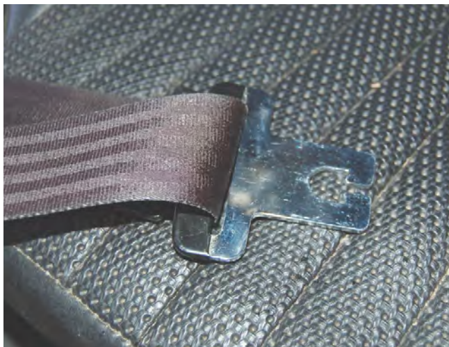
A later seat belt tongue – a totally different shape to the early ones.
