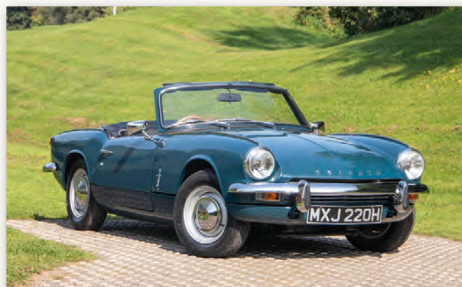
For 1967, the front bumper was raised to give a lower look to the front end, which was revised with a full width grille and under-bumper indicators/side lights. A larger version of the SC engine was also introduced.
