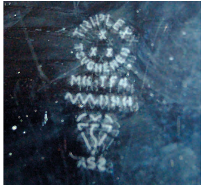
Pre-1969 Triplex logo – this shows a 1968 glass (large dot under the 'E') but the quarter is not clear – is that a dot over the 'T' or just a mark in the screen ?
