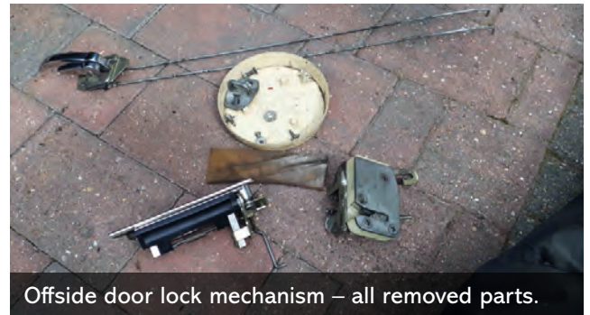
Outer door handle inner mechanism.
