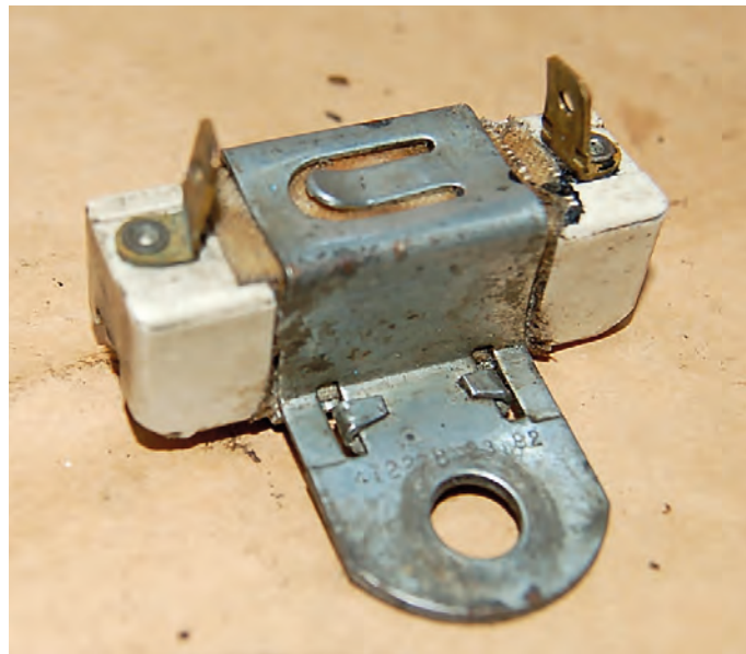
A ballast resistor (part no. 134176). Quite a complicated item just to provide a fixed resistance in a circuit.
