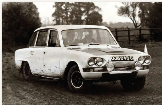
I'll leave you this month with a photo of one of the 2.5PI rally cars. Although this car was used in the Austrian and Scottish Rallies in 1969, this photo was probably taken during its later life as a test and practice car for the 1970 RAC Rally. The matt black bonnet was not for team identity but was to prevent obtrusive reflections during night rallies.
