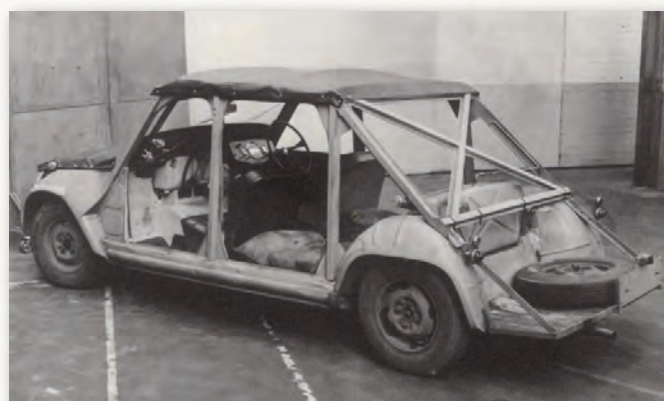
The 'Birdcage', as it was known, with which the Engineering Department carried out the initial endurance testing for the new large saloon. Believe it or not, this was a road test vehicle and spent not a few hours being driven over the company's normal test routes
