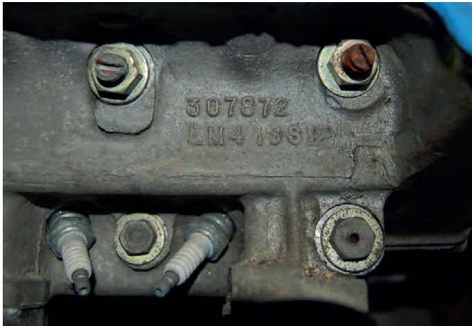
A prototype cylinder head showing that it has the same casting number as the early production heads but was cast in LM4 not LM25.
