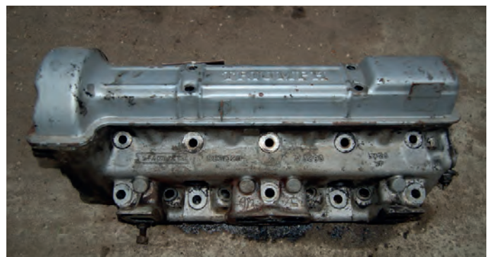
A Mk2 LH cylinder head. The characters cast into the head along the central land are 'Stanpart', '88313210', 'V3293' and 'LM25 WP'.
