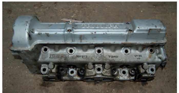
A Mk1 LH cylinder head. The characters cast into the head along the central land are 'Stanpart', '307872', 'V3143' and 'LM25 WP'.
