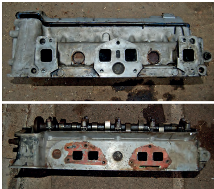
The five core plugs in the heads, three on the exhaust side and two on the inlet manifold side.
