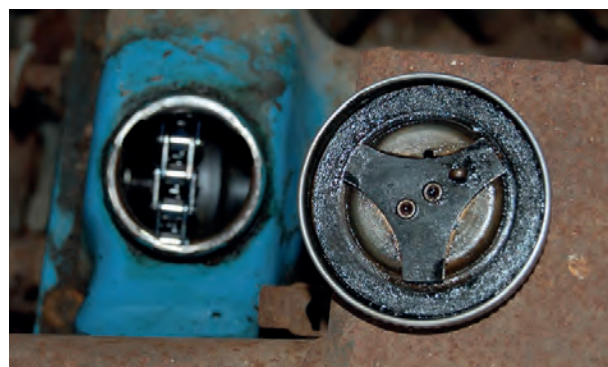
A '3-ear' filler cap from an early engine (LF 17). The finish of the cap is chrome whereas later caps were passivated.
