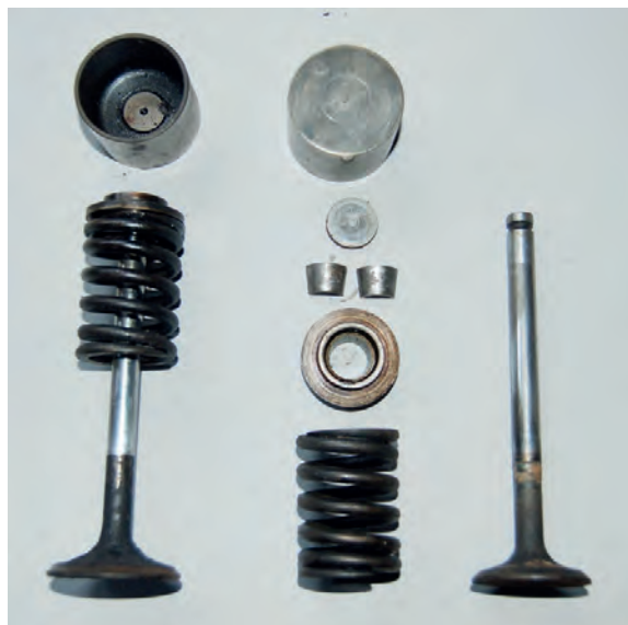
Valves, springs, collars, collets, shims and pallets as they come out of the engine. The inlet valve is the slightly larger one on the left, the shim being stuck to the inside of the pallet.
