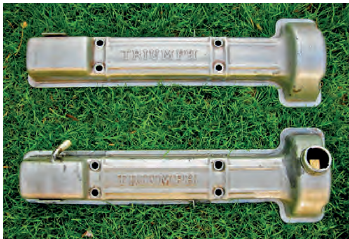
'Triumph' is the same on both cam covers but the top one is upside down as it should be readable from the nearside of the car. It was put in the jig back to front when it was stamped.
