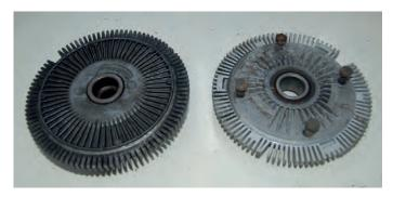
The back (engine side) of an early Torquatrol unit (left) and that of a later unit (right) showing that they are very different and that it is only the later unit which has the fixing bolts passing right through the unit. Why do all my Torquatrol units seem to have two vane ends missing?
