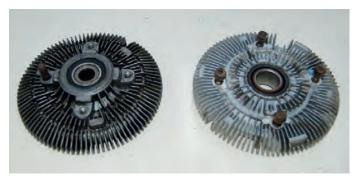
The front faces of the units shown in the last photo. You can see that the 'integral bolts' in the early one are actually studs (one is still in place) whereas the later one uses through bolts on a different diameter.
