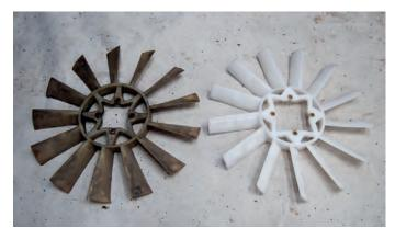
An early (dirty) and a late (clean) fan – but I don't know which early fan. It came out of a very early car but that is no guarantee that it is the very first fan type. The centres are different, as are the blade shapes and although the securing holes look to be in the same positions, they are spaced on a larger PCD than the newer fan.
