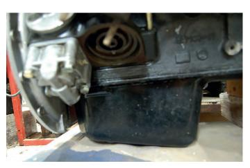
A (very) early sump without the bracket for stiffening the transmission housing – although this engine has a later housing with the lug cast in. Note the more complicated machining than normal in the oil filter housing. I will touch on this in the December catch-up
