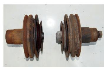
The damper and power steering pulley assembly with the short spigot version on the left and the long spigot version on the right.
