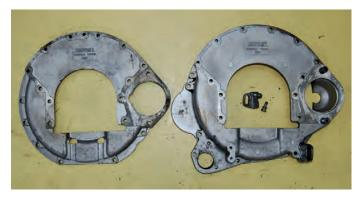
An early transmission adaptor (on the left) and a later clutch housing (on the right). The differences are obvious in the flesh as, although you cannot see this in the photo, the right hand one is a much deeper casting and it has extra flanges on its left hand side for the slave cylinder and for a cover to the clutch mechanism.
