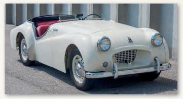
A 1954 TR2 for comparison with the picture below. This looks like a 'long door' example and, following complaints about the door bottom hitting the kerb when opened, Triumph cut 4in off the bottoms (from TS 4002).
