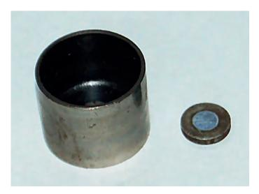
On the left is a tappet or cam bucket and on the right is a pallet or shim. So, a shim is a pallet and the part which I called a pallet is a tappet or cam bucket. If you google 'what is a pallet in an engine' there is no answer other than 'a wooden thing to deliver it on' so I made an assumption based on the description of a dismantling process – and I got it wrong. Sorry.
