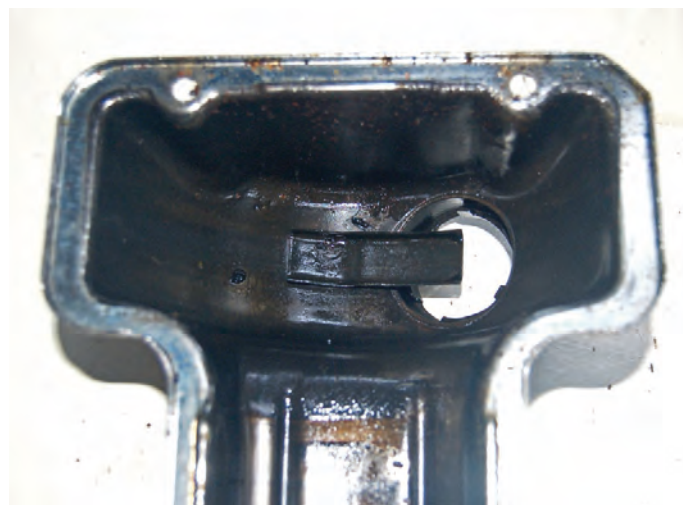
The small splash guard spot welded into the RH cam cover immediately below the oil filler hole.
