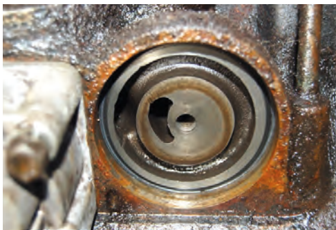
Later oil filter housing casting with a smaller inner oilway.
