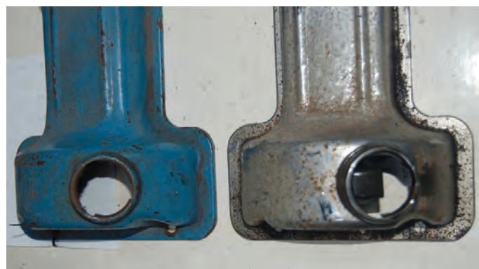
As you can see, no guard under the blue cam cover oil filler hole (on the left).
