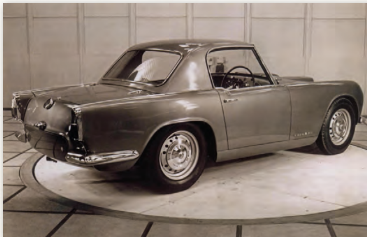
Rear view of the original Michelotti Zest prototype (X614) complete with Herald coupe style hard top.
