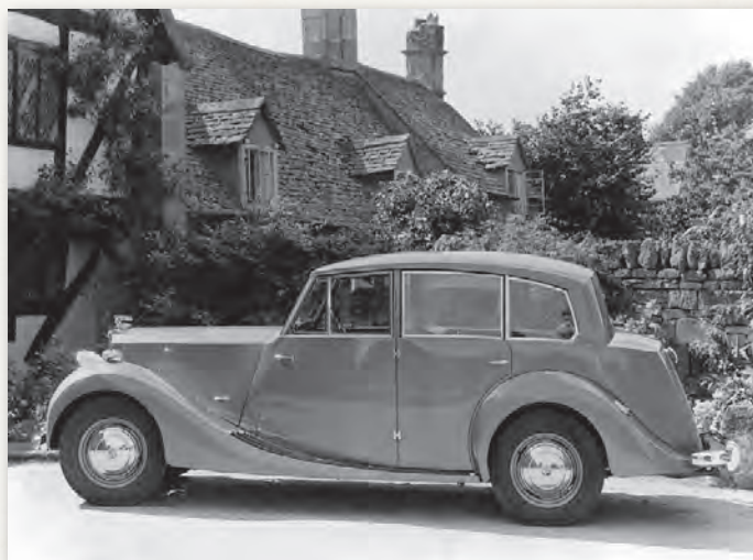
Side view of an 1800 Town & Country Saloon showing the large flat panels with their sharp panel joints – all except for the flowing wings.
