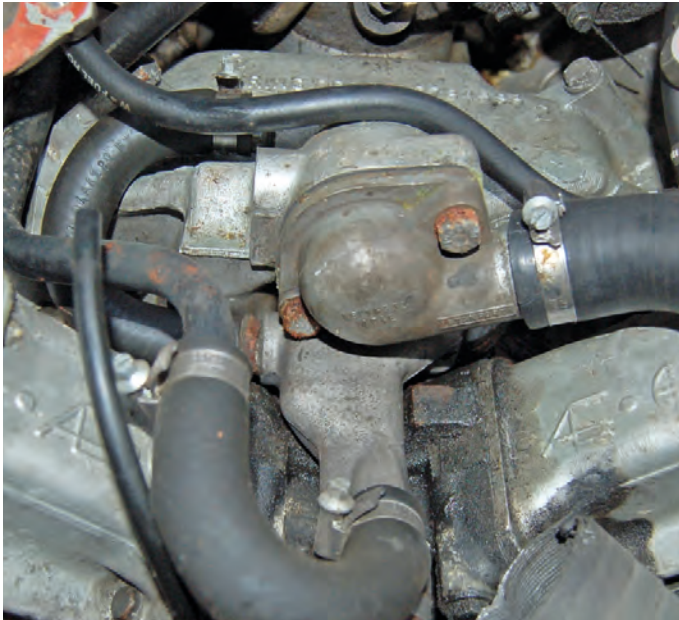
A later engine layout with a thinner thermostat cover flange. The bypass hose now feeds from the back of the thermostat housing (seen under the small black pipe towards the top of the photo) to the side of the water pump cover, whereas the spigot on the top of the water pump is angled and receives water from the heater hose.
