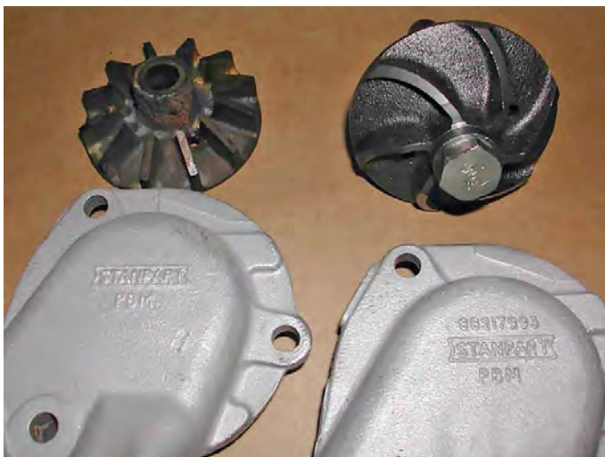
6 vane and 12 vane pump impellers and pump covers. The impellers are obviously totally different, the covers are also different as the angle of the inner housing is steeper for the 6-vane version – luckily, 6 vane covers have the part number (with an 88 in front of it) cast into top surface so that you can easily tell the difference. Photo stolen from our forum pages – sorry 'Staggering About' but it is a particularly good photo and I couldn't resist.
