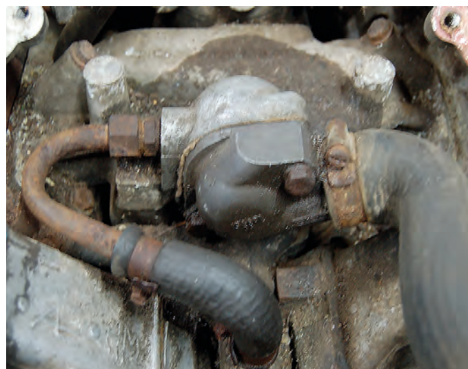
An early engine equipped with the 'thicker' thermostat cover and a metal bypass pipe feeding into the top of the vertical spigot on the top of the water pump.
