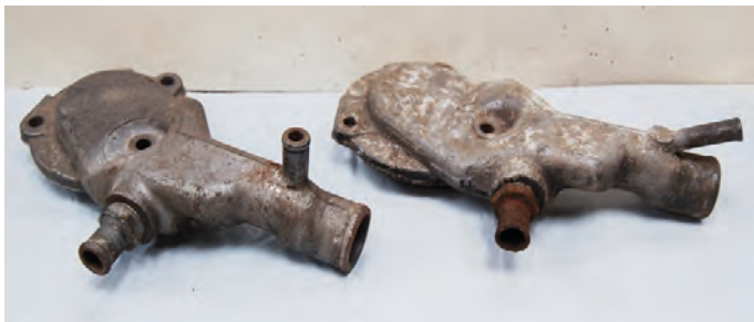
The two different water pump covers used with the six vane pump for UK and European market Stags.
