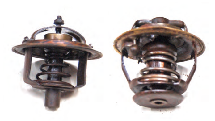
The two thermostat types used in Stag. The early one without a foot for use with the early inlet manifold (left) and the later one with a 'foot' which blocks off the bypass exit in the later inlet manifold when the thermostat opens.
