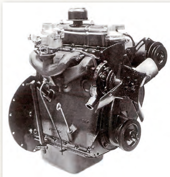
The Small Car (SC) engine of 1951. Inlet and exhaust this side, everything electrical on the other side.
