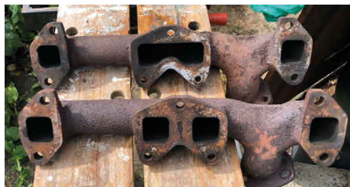
The change in exhaust manifold which you will rarely see – the very early manifolds had a centre wall in the twinned middle exhaust flanges. (Photo: Aidan Platten)
