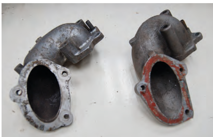
The early (left) and the late (right) carburettor elbows. Note the much smaller bolt bosses on the early one. There were other differences as the early one is a smoother finish and I would suggest that they moved from a diecast to a sand cast elbow, the sand cast item being slightly rougher.
