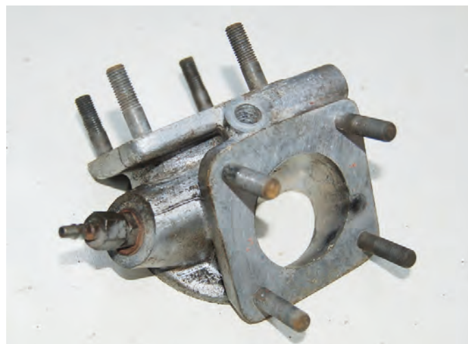
A carburettor pedestal. The one-way valve is screwed into the boss under the carburettors.
