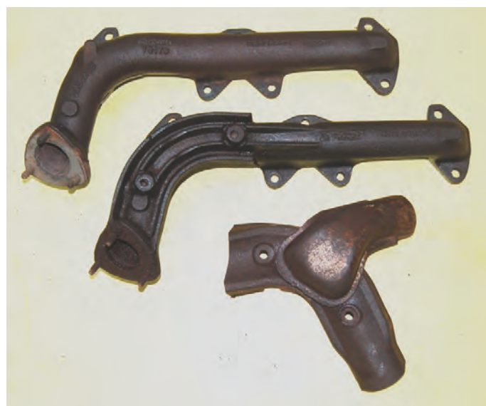
An early LH exhaust manifold (top) and the later manifold (centre) with the cowl used to take hot air to the air filter box via the 'elephant's trunk'.
