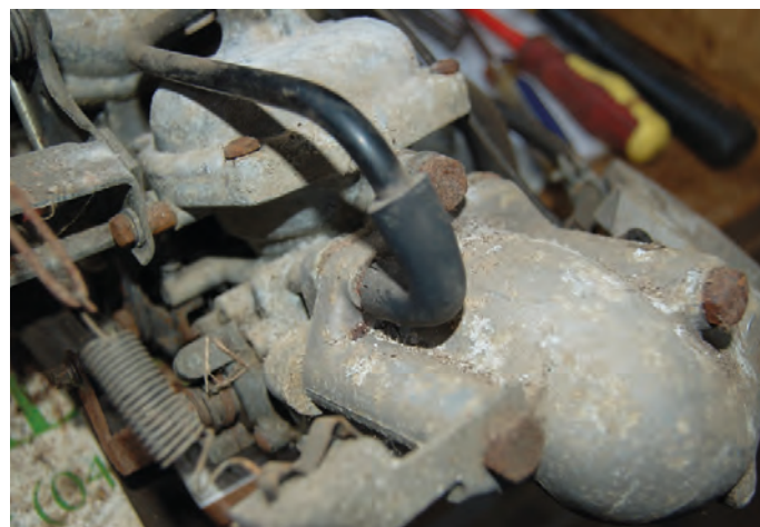
This is the early 2S carburettor with the simple vent back to the air cleaner.
