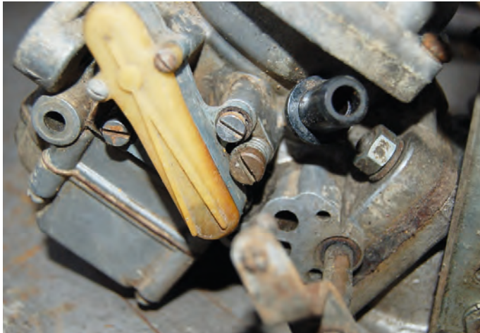
The idle trimming screw is slap bang in the centre of this photo, next to the bottom of the temperature compensator.
