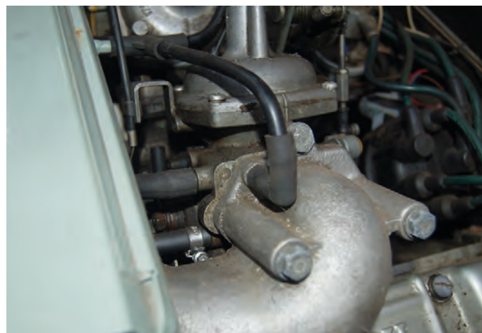
Whereas the 2SEV carburettors have a second vent pipe (to the left of the original pipe) which operates when the engine is stopped or idling.
