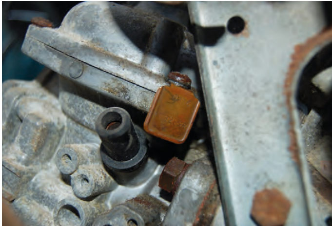
Location of the brass tags on the carburettors. This one says '0396' and '3289R' which indicates that it is a CD2S from 1970-71 (see table below).
