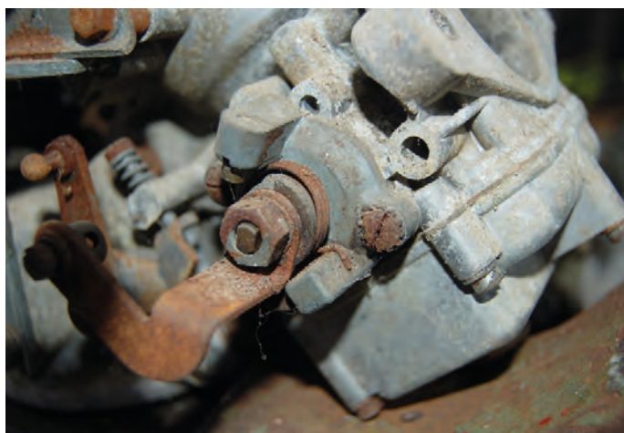
The cold start valve (in the centre of the photo) on this rather crusty carburettor is held on by a simple screw either side and is operated by the choke cable bracket.
