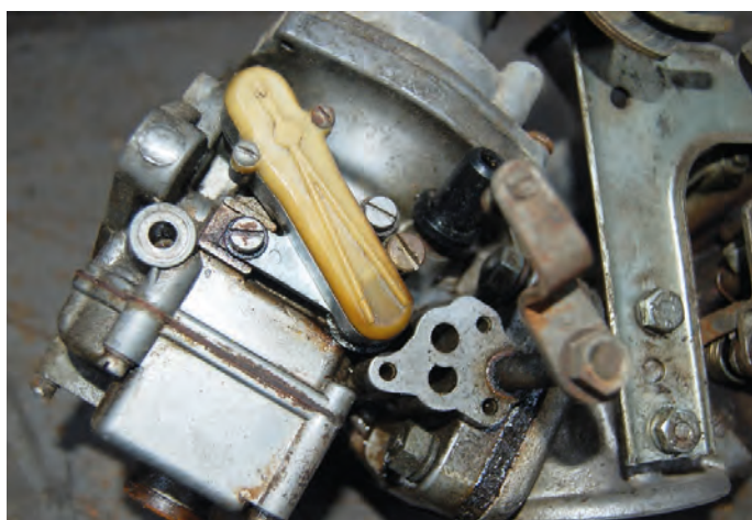
The temperature compensator is the long, white plastic moulding on the side of the carburettor.
