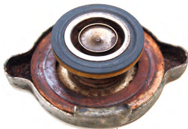
An early radiator cap with the central return valve and space around it for the returning water to flow back through.
