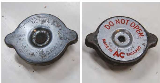
An early 13psi radiator cap (right) and a much later 20psi radiator cap (left). I believe that the generic markings on the later cap shows it to be one of the GRC124 caps.
